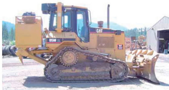
Figura 21 Tractor de cadenas con depósito y bomba, tipo Pumpercat. Foto: "Yellow book" Mechanized Equipment for Fuel and Fire Operations.2009.
