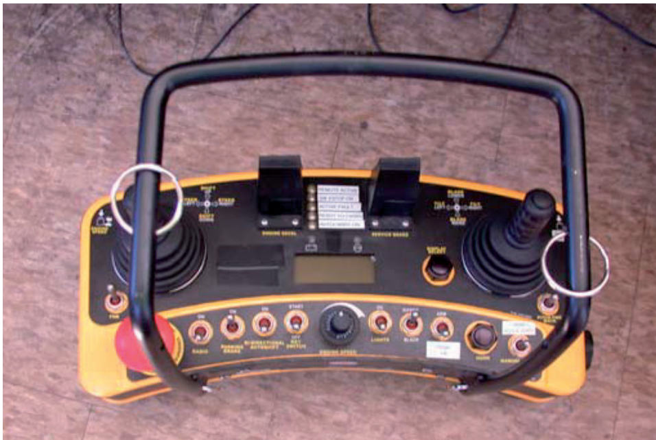
Figura 194 Mando del control remoto. Remote vision system for dozer in stockpiles. Foto: William H. Schiffbauer.
