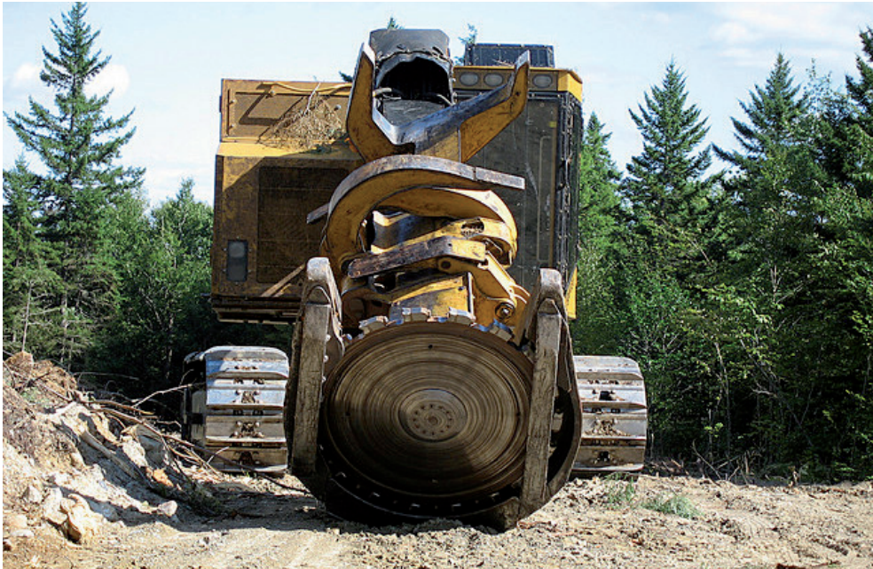
Figura 13 Taladora de sierra de disco sobre retroexcavadora. Foto: "Yellow book" Mechanized Equipment for Fuel and Fire Operations. 2009.
