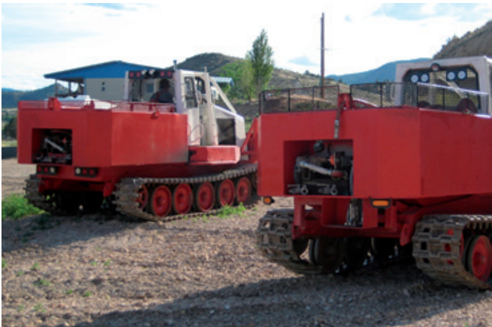
Figura 23 Tractor de cadenas flexibles con depósito y bomba. Foto: "Yellow book" Mechanized Equipment for Fuel and Fire Operations. 2009.
