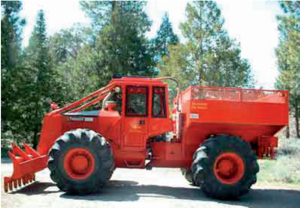
Figura 22 Skidder con depósito y bomba. Foto: "Yellow book" Mechanized Equipment for Fuel and Fire Operations. 2009.
