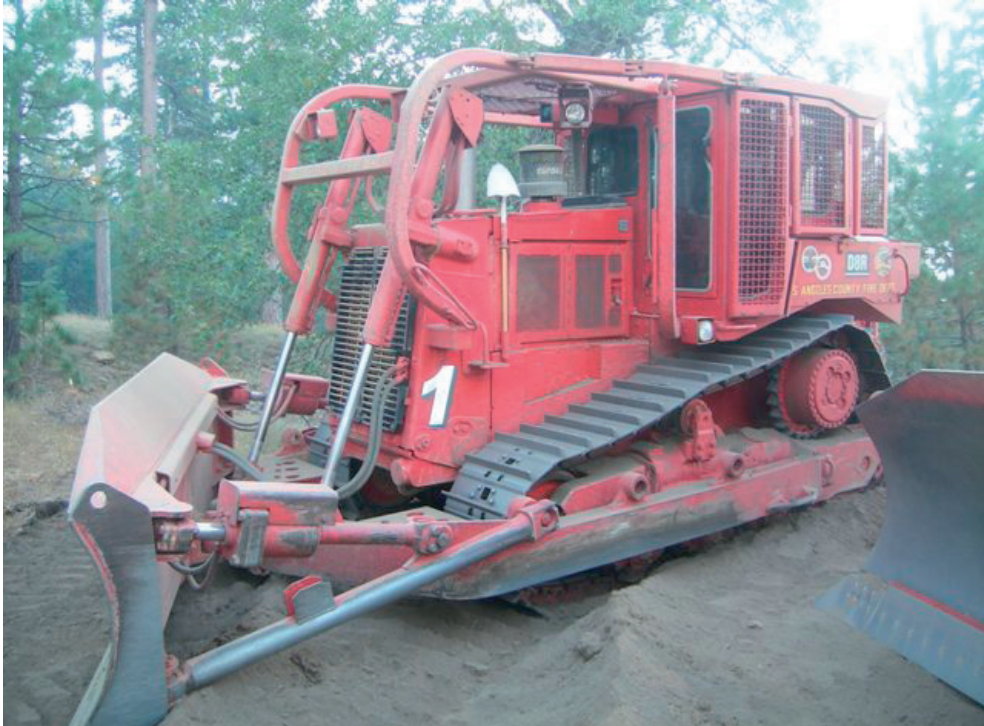
Figura 133 Protecciones especiales en Bulldozer CAT D8R de Los Angeles County Fire Department. Foto: California Dozer Operator's Group.
